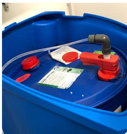
Fig. 2: A keg tap opens the disinfectant drum, meaning that the operator does not work with an open drum at any time.
